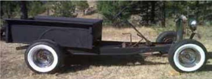
1932 Ford pickup rolling chassis includes: pickup bed; four 15" chrome reverse wheels; original 'K' member and cross members; front fender braces; radiator; headlight bar; and steering box and column with original key in column lock. The torque tube and rear end were chromed in the 1960's Price: \$3500
